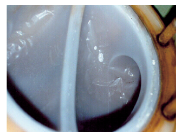
PVDF/Blister is observed (Electrolysis Plant/ Return Brine 88°C, 0.3MPa, after 5years service)
